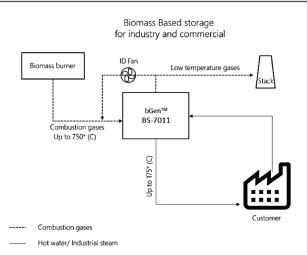
The BS-7011 can be activated in different working points. The following table specifies such sample points. One can use it to maximize power or to maximize capacity. The unit maximum delivery is 1 ton of steam.
